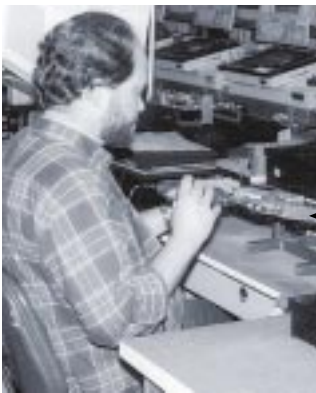
A light-weight, adjustable fixture holds the motherboard during inspection or repair.
