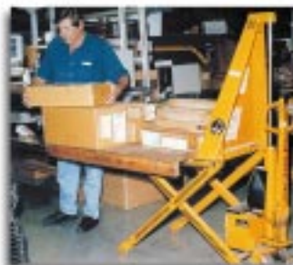
▲ Scissors lift provides a portable, height-adjustable workstation
